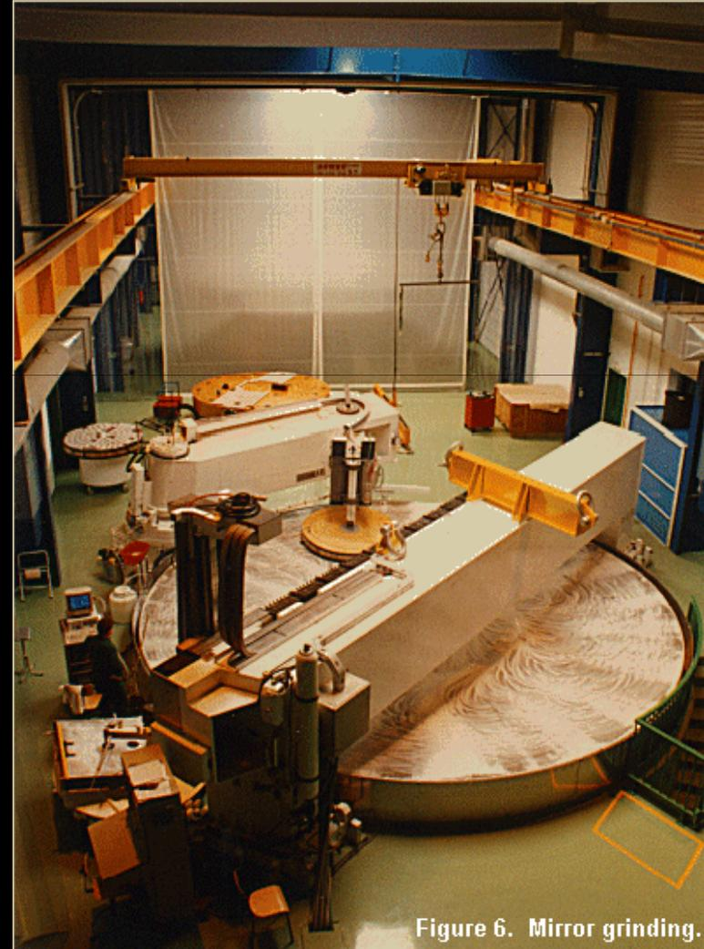
Figure 6. Mirror grinding.
