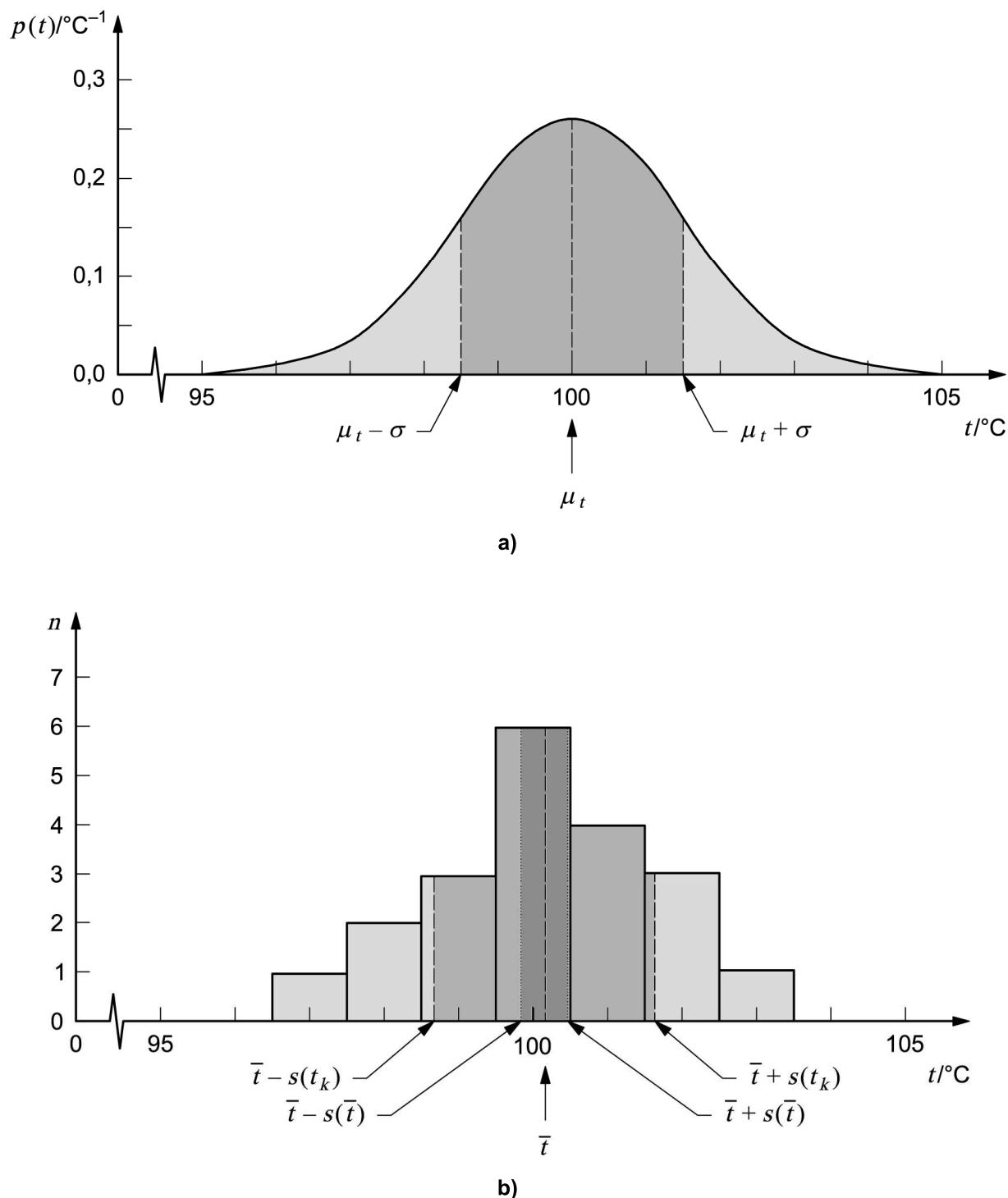
**Figure 1 — Graphical illustration of evaluating the standard uncertainty of an input quantity from repeated observations**
